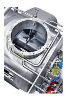
Black/white separation can prevent the spread of contamination. In technical terms, this means, for example, spatially separating the motor for driving a mixer or other process engineering machine from the machine itself.
