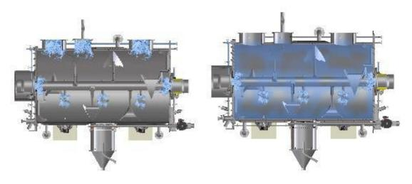
Whether washing-in-place, cleaning-in-place or sterilisation-in-place: Hygienic execution is only guaranteed if all points in the machine can be reached and wetted by cleaning agents and disinfectants without obstruction.
