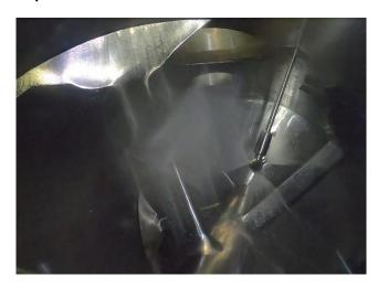
Rotating flat fan cleaning nozzle in a 10.000 l Lödige Ploughshare®-Mixer in operation. (Source: Lödige Process Technology)
