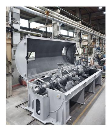
**Fig. at the top:** View inside the mixing drum **Fig. at the bottom:** Mixing drum getting closed by using a crane
