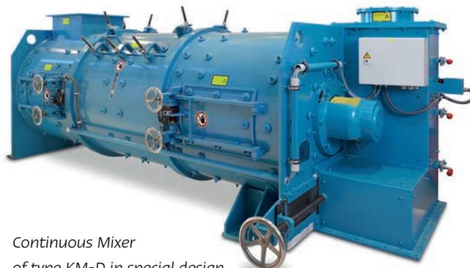
*Continuous Mixer of type KM-D in special design with exchangeable anti-wear lining*
