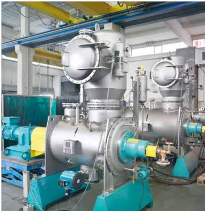
DRUVATHERM® type VT 300 Vacuum Shovel Dryer, with heated shaft
