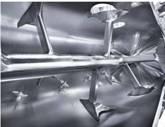
Welded mixing unit in hygienic design
