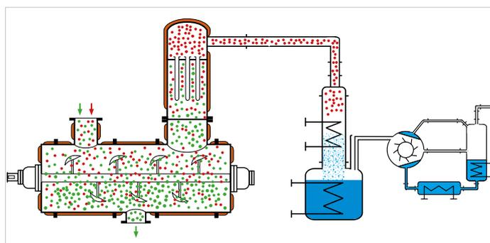
Principle of the vacuum shovel dryer DRUVATHERM®
