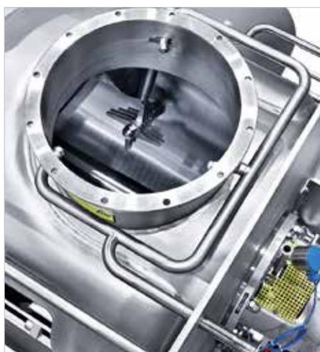
Cleaning nozzles for the WIP cleaning process
