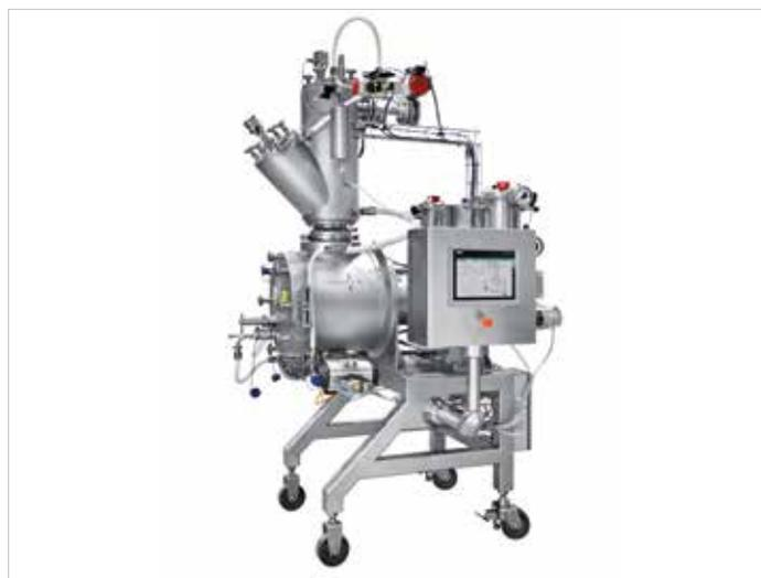
Vacuum shovel dryer DRUVATHERM® type DVT 50 as the pilot plant for research and development
