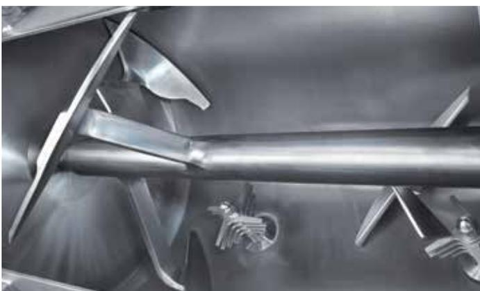
Fixed welded mixing unit in hygienic design
