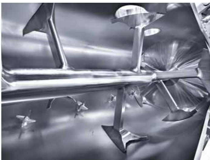
Welded mixing unit in hygienic design
