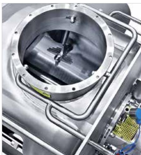
Cleaning nozzles for the WIP cleaning process
