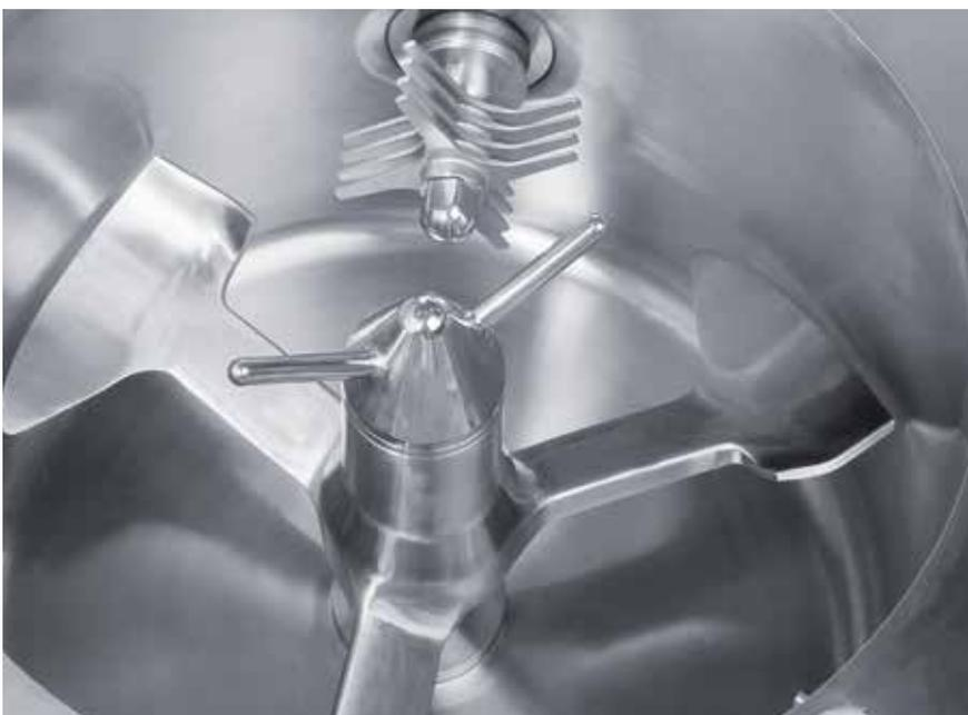
Mixing tool with tool lifting unit
