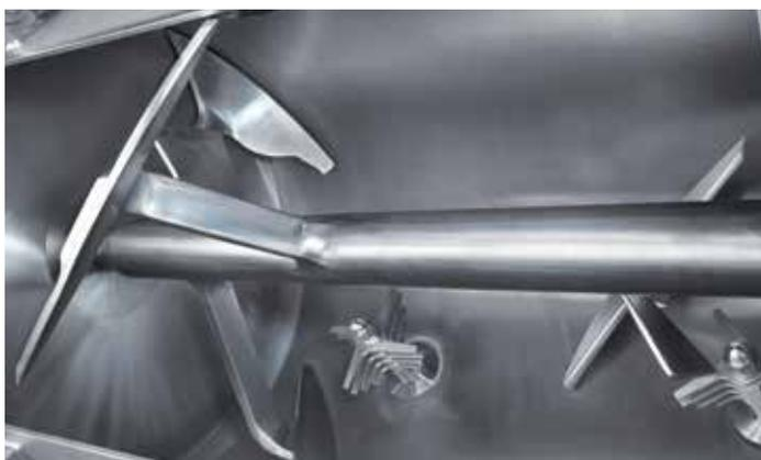
Fixed welded mixing unit in hygienic design
