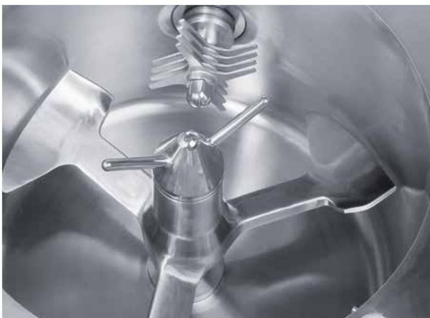
Mixing tool with tool lifting unit
