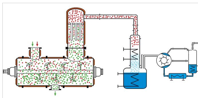
Principle of the vacuum shovel dryer DRUVATHERM®
