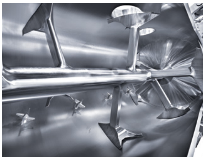
Welded mixing unit in hygienic design
