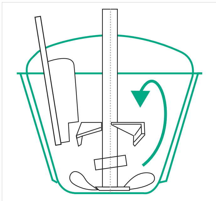
Mixing principle of the wet mixer NOHK
