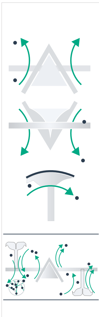
Mixing principle of the Lödige Ploughshare® Mixer
