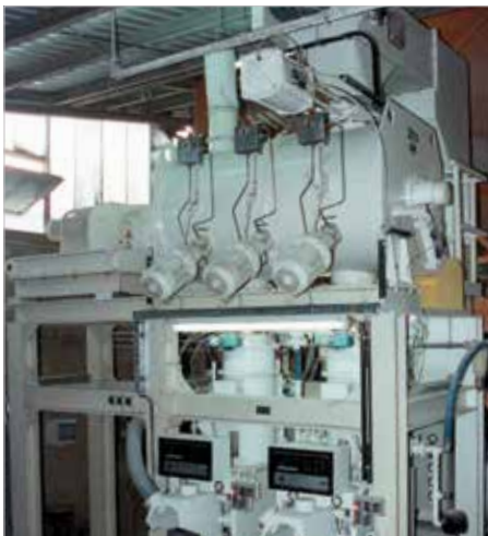
Ploughshare® Mixer with automatic bag filling
