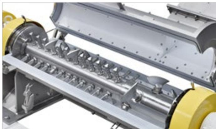
Liquid components can be added through the mixing tools in case of aqueous liquids
